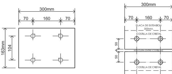
BARRENO PASADO PARA PLACA DE EXTENSION 300MM. EN CRISTAL TEMPLADO MONOLITICO DE 19mm.
